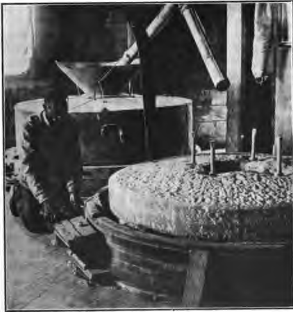
FIG. 8.—Large stones for hulling rice, and removing chaff. Savannah, Ga. (Copyright by Keystone View Co.)
